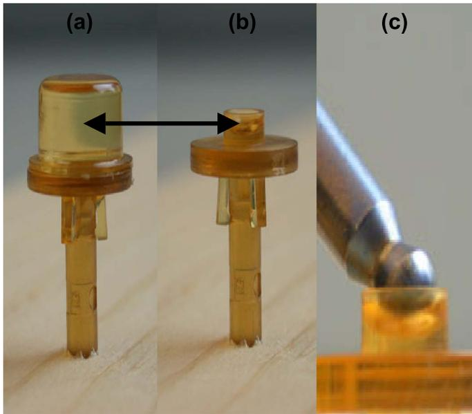
Fig. 2. Radiographic marker (a) and physical marker (b), each mounted on the same post. In (c), the spherical tip of a tracked probe is shown in contact with the hemispherical divot of the marker in (b). The arrows point to the centroid of the radiographic marker and the center of the divot in the physical marker.
