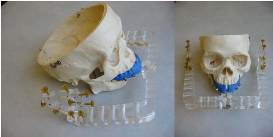
Fig. 1. Fiducial frame (constructed of plexiglass) mounted to cadaveric dentition using LADS. Fiducial markers are shown surrounding each temporal bone.
